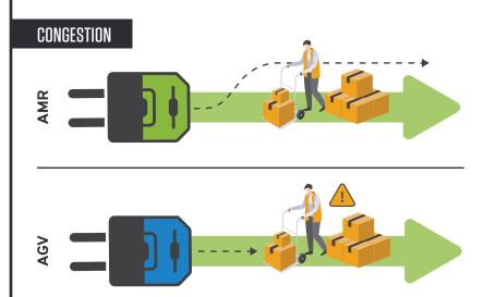
By comparison, because an AMR is a Path-Planning robot, it does not need to adhere to a fixed route and can adjust its path to provide more space to the staged pallets near the path, allowing both the robot to drive at maximum speeds and still leaving ample room for people to safely move about.
