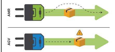
Path Planning allows an AMR to adjust routing and navigate independently around obstacles without stopping and requiring assistance from workers.
