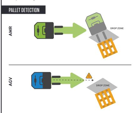
AMRs make use of detection – that is, positive confirmation via onboard sensors – to determine if the pallet is there before they attempt the pickup. If the pallet is askew, or slightly out of the drop zone, the robot will be able to identify it. If the right pallet is not where the AMR anticipated it should be, it will move to the next drop area and search again.
