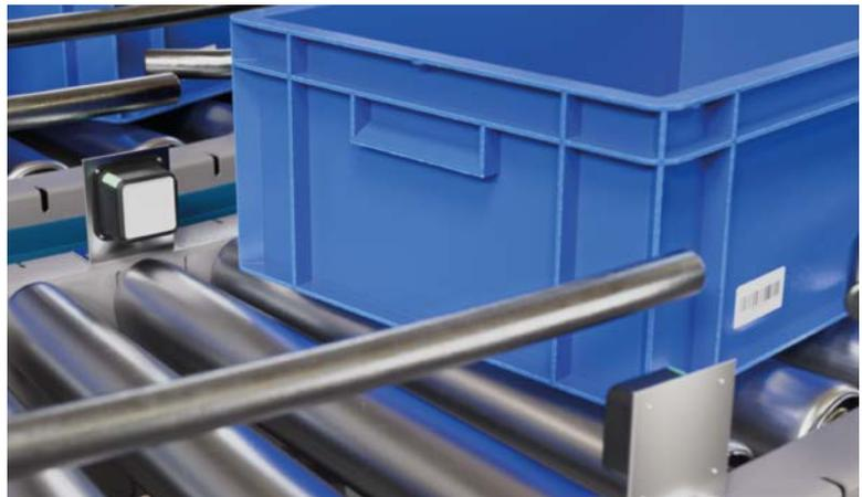
Barcodes are a relatively inexpensive method of marking items but it is difficult to automate barcode reading in high volumes.
