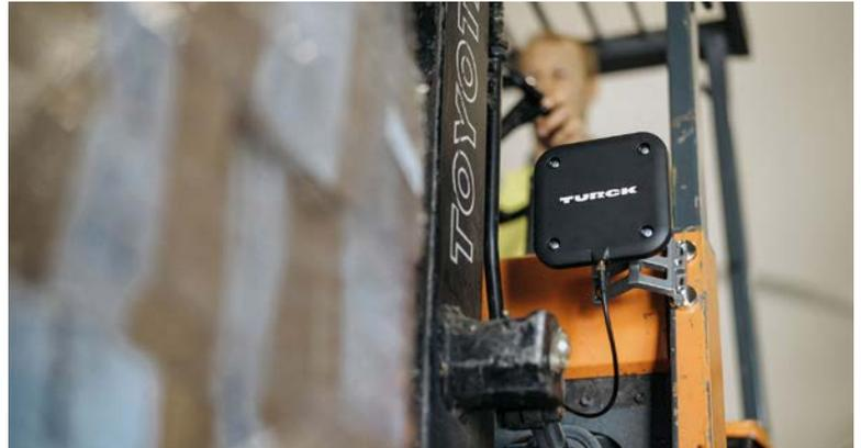
Forklift trucks equipped with RFID readers achieve high reliability and speed in identifying and tracking pallets, and containers.
