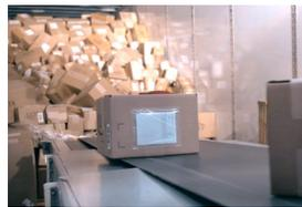
**Unloading trailers** - Using extendable conveyor that reaches completely inside a trailer can allow a worker to simply lift, turn and place parcels at an ergonomic height.
