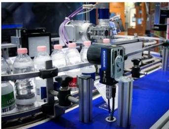
Machine vision is an image-based technology that is used for inspection and analysis, vital when you want to make sure the correct components are in the correct place in the correct order. The smart camera can inspect the “human readable” code next to the barcode and aids in pattern identification, flexible packaging – such as pallets with different products – and image archiving.
