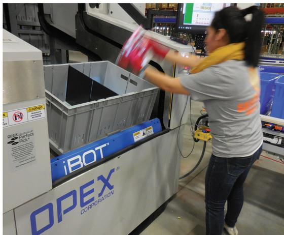
Once the pick is completed into an order tote via pick-to-light, the product tote is taken away and the next tote is immediately presented. This allows workers to typically pick over 400 items an hour, compared with the 200 items that workers in the facility's pick module select, so it is twice as productive. Orders can now be completed within 30 minute of being inducted, which allows Newegg to meet its same-day shipping goals.
