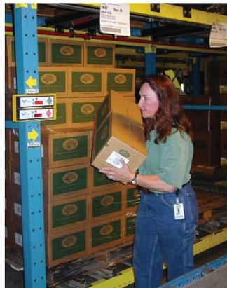
Full cases of coffee are selected in pick tunnels using pick-to-light technology. These are placed onto conveyor belts that run through the tunnels.
