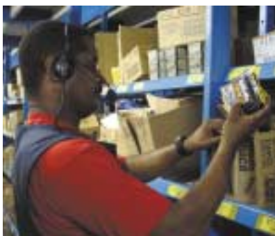
A voice-directed system guides a worker in selecting repack items at Associated Grocers. The system relays instructions using a headset and the worker responds by speaking into his microphone. The interaction between system and worker results in hands-free picking with very high accuracy.
